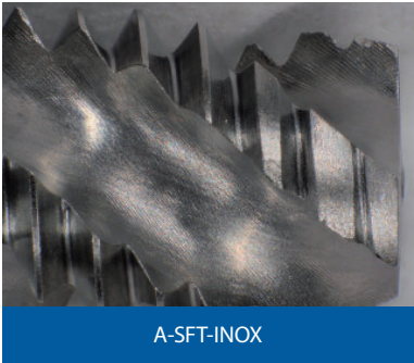
Cutting edge after tapping 1.000 holes
